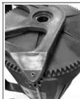
6. Move the 4" hole in the cradle so it is over the 4" bearing in the drum, and press down firmly with the flat of the hand so that the cradle locks onto the drum (use a rubber mallet if necessary).
