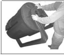
3. The handle is installed onto the shaft in the factory. To disconnect the handle, use the allen key (provided in the kit) to remove the set screw from the handle assembly. Pull and/or twist the handle from the shaft. Note the black mark on the shaft. This should be positioned near where the set screw fastens the handle to the shaft and should be in the same position when the handle is re-installed.
