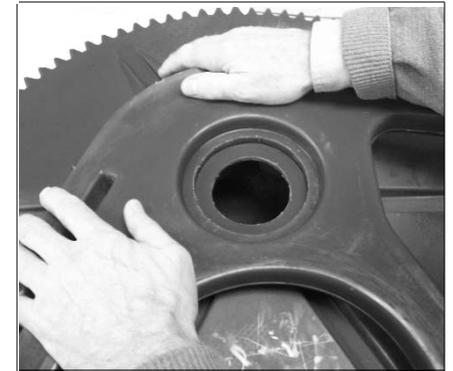
7. Place a 1/2" washer onto the shaft so it is up against the outside of the cradle, and then secure by placing the cotter pin through the hole at the end of the shaft. Use pliers to bend the legs of the cotter pin so the pin is secured.
