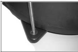
5. Insert a 1/2" washer over the shaft to rest against the gear. Pry the cradle away from the large gear end of the drum until the shaft can be inserted into the hole on the cradle and the small gear is positioned against the large gear on the drum.
