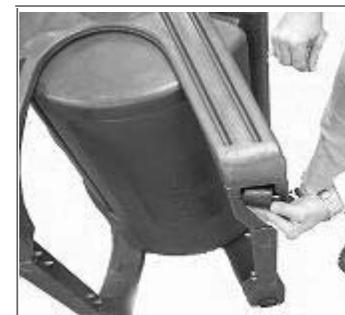
9. Place a 1/2" washer onto the shaft at the output end, then push the handle on to the shaft lining up the black mark near the hole in the shaft with the hole in the top of the handle. Insert the set screw into the pre-drilled hole in the handle. Screw in the set screw using the Allen Key supplied until the set screw is completely inside of the handle.
